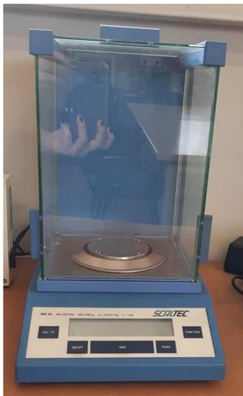
Figura 32. Balanza SCALTEC SBC22
