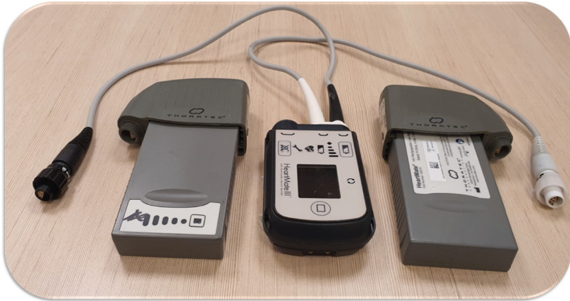
Figure 2. The extracorporeal parts of the HeartMate 3 system including batteries and controller.
