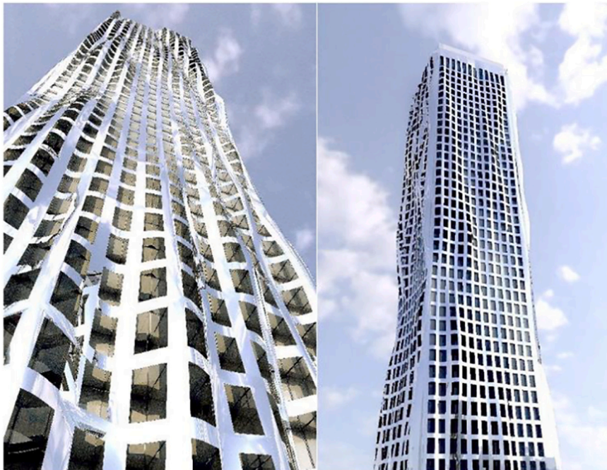
Fig. 11. Tower design resembling the Beekman Tower generated by a GA and rendered in Vray. Pazos, 2017.
