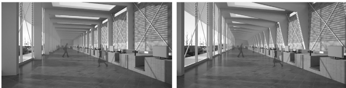
Fig. 2. Two options for the design of the lateral and gravity structural system for an airport terminal: (left) a standard rigid frame and (right) a shaped rigid frame. The shaped frame uses a similar amount of material and creates a more architecturally expressive interior space. Mueller and Ochsendorf, 2015.
