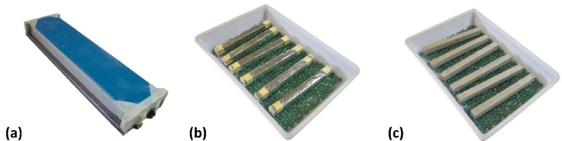
Fig. 6. Curing conditions of specimens for determining mortar strain: (a) in moulds, (b) in sealed condition (b) and (c) in air drying environment.
