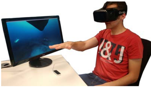
Figure 1: A pilot tele-operating a ROV using a VR headset for achieving an immersive experience and sending commands using gesture recognition.
