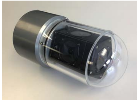
(b) The omnidirectional underwater camera used for the survey.
