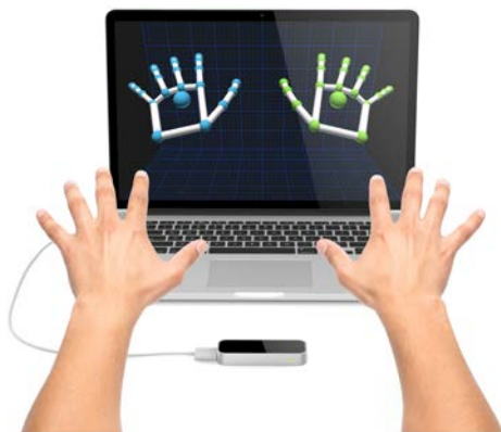
Figure 4: Hands motion being tracked by the Leap Motion Device.
