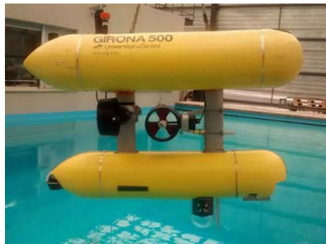
(a) The omnidirectional camera integrated with the Girona500 AUV.
