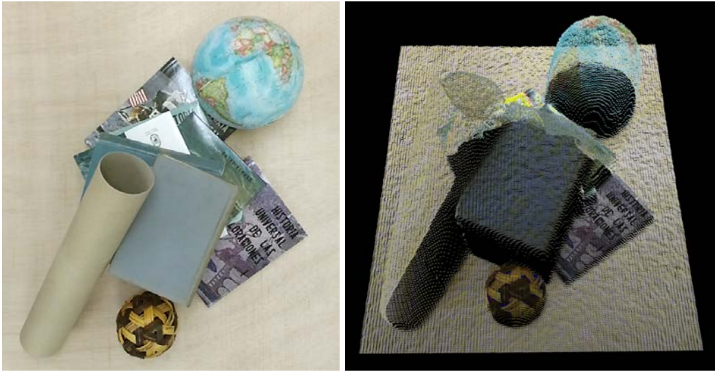
Figure 2: A scene used as an example of a cluttered pile of man-made objects (left), and the depth map acquired using a Kinect 2 sensor (right).
