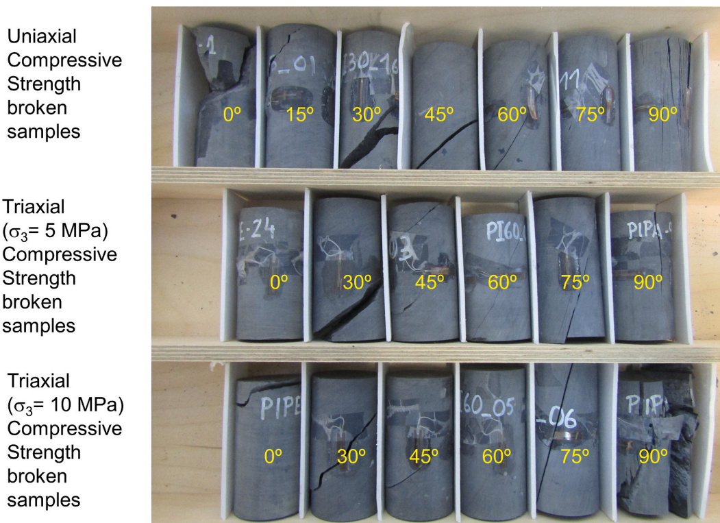
Fig. 8. Photograph of representative slate samples after testing for various foliation inclinations and confinements.
