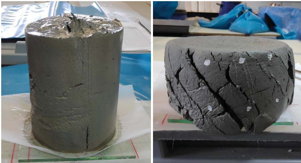
Figure 42. Fresh mortars before and after performing green strength test.
