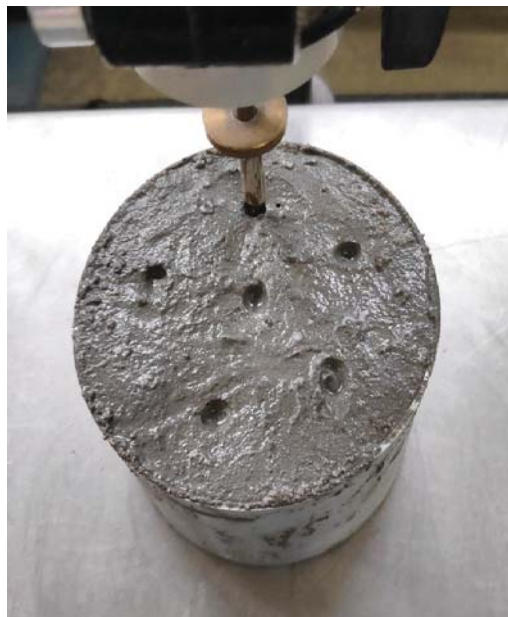
Figure 18. Fresh mortar after open time test.
