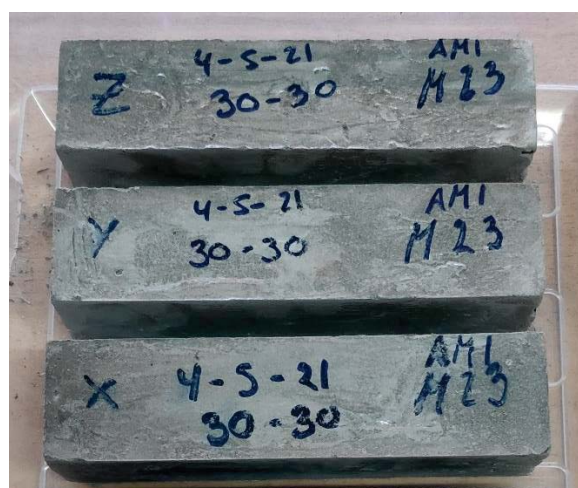
Figure 24. Mortar test specimens at age 1 day old.
