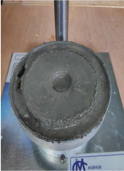
Figure 15. Fresh mortar after open time test.
