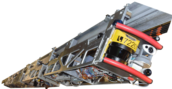
Figure 2: The Train Inspection Monorail hanging from the LHC's roof rail
