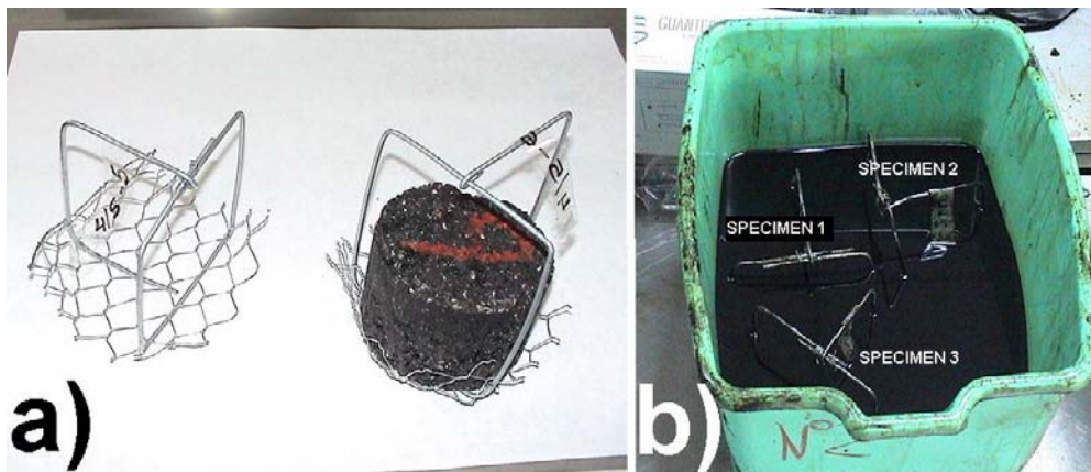
FIGURE 2. a) Metal basket and specimen inside the basket. b) Three specimens in the fuel bath.
