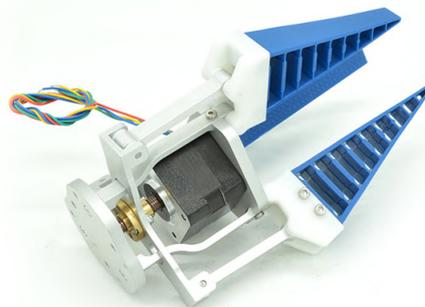
**Figura 8.10** – Gripper flexible final
