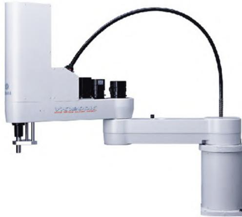
**Figura 3.9** – Robot SCARA
