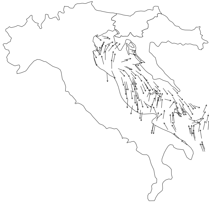
Figure 4.5: Random sample of 150 wave directions in the Adriatic Sea area on April 2, 2010 at 6am during a calm period.
