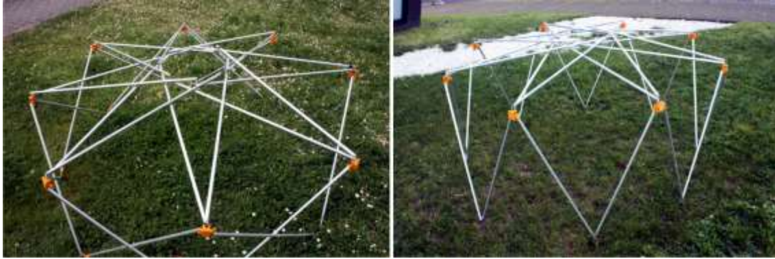
Figure 11: Models used to test kinematic compatibility. Type a) and b) yurts.
