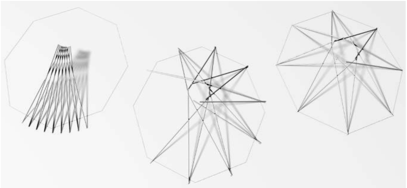
Figure 4: Diagram showing how the roof covering of the yurt is deployed.
