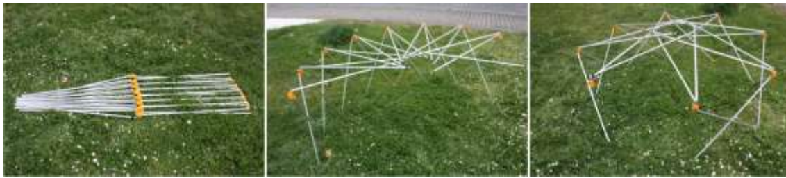
Figure 13: Radial deployment of a model of a type a) yurt.
