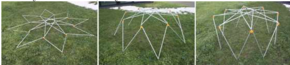
Figure 14: Deployment by raising of a model of a type b) yurt
