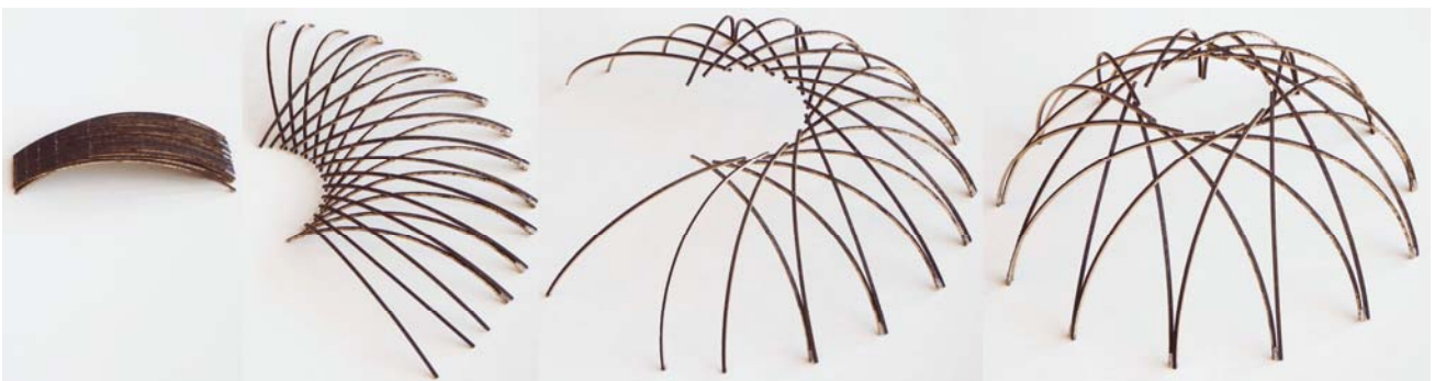
Figure 16: Deployment process with vertical axes
