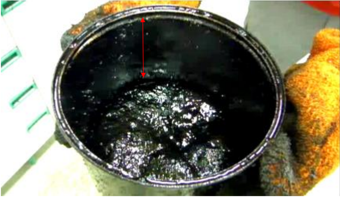
Figure 5. Bitumen with 20% of industrial waste: a) at the beginning of the mixing process and b) after 5 s of the beginning of the mixing process
