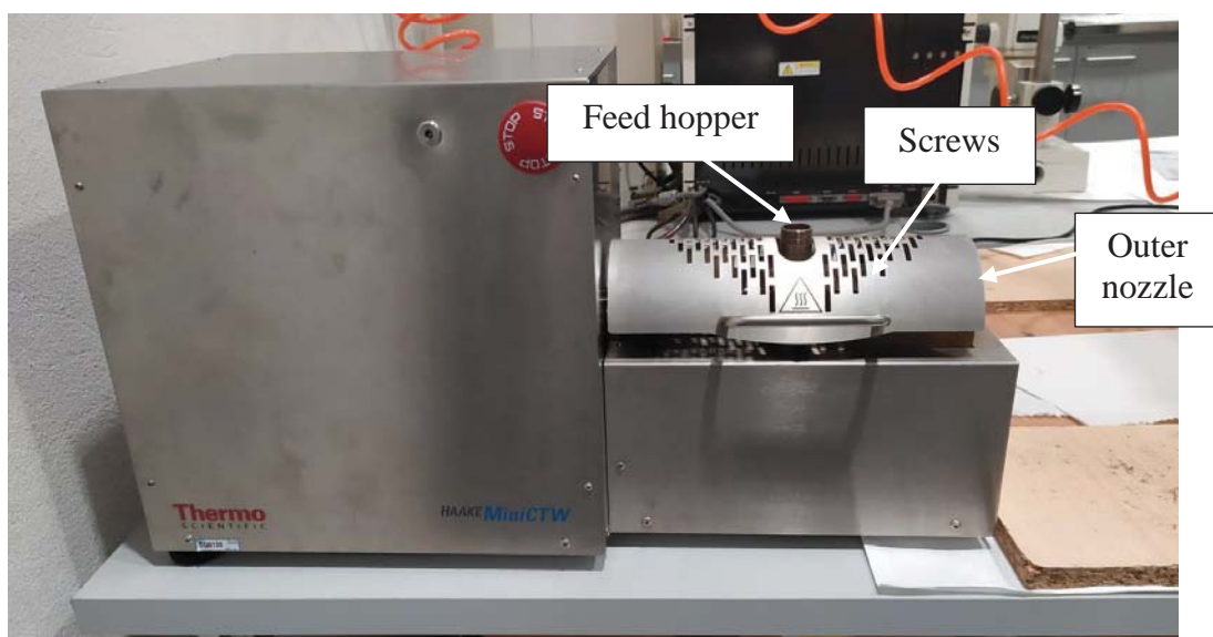
Image 1: Mini extrusion machine from CETIM.
