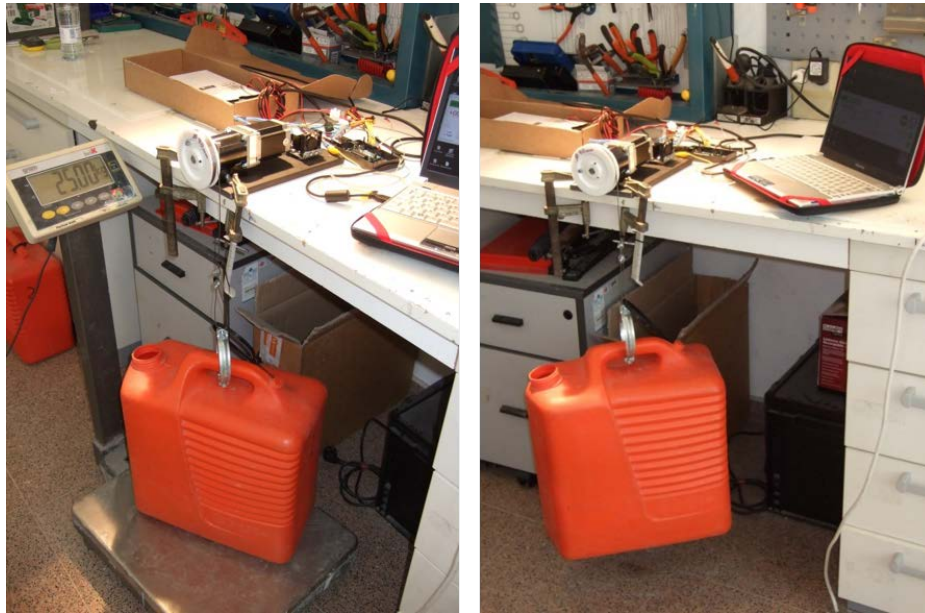
Figure B.8: Elements used to perform preliminary load tests with the motor/gearhead assembly.
