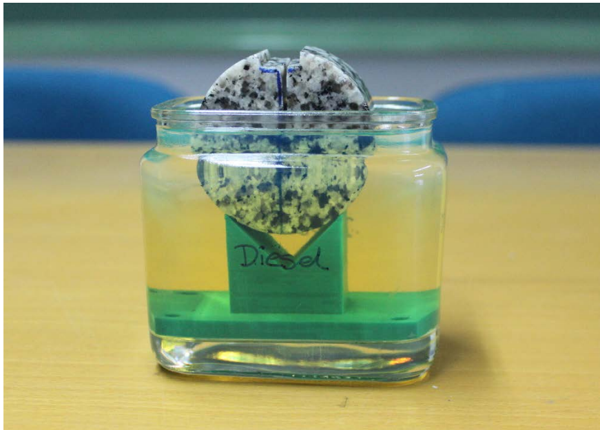
Figure C.2: Prepared specimen of Blanco Mera granite immersed in diesel fuel before testing.
