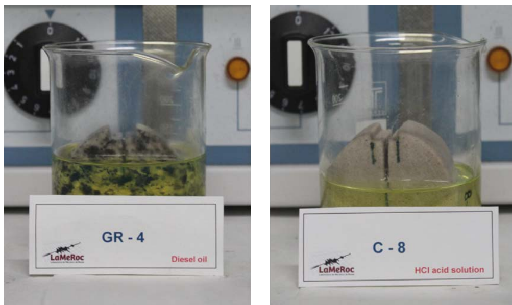
Figure C.1: p CT specimens of Blanco Mera granite (left) and Corvio sandstone (right) immersed in diesel fuel and HCl solution, respectively.
