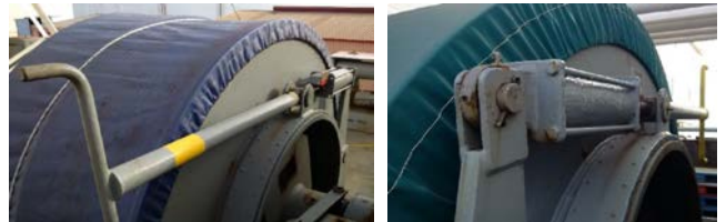
Figure 7. Spring-applied band brake with manual release of LNG Tanker "Excelsior".
