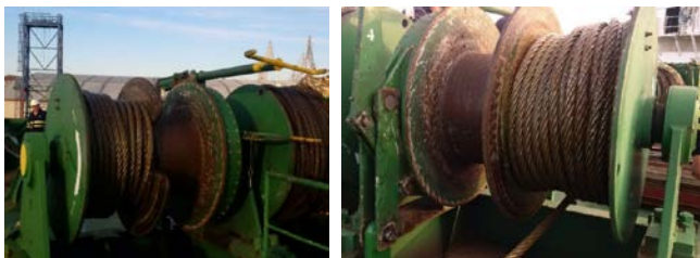
Figure 12. Mooring winch of split drum type dotted with spring-applied band brake with manual release where the brake test was performed. The necessary wire rope was spooled off to have enough free space.
