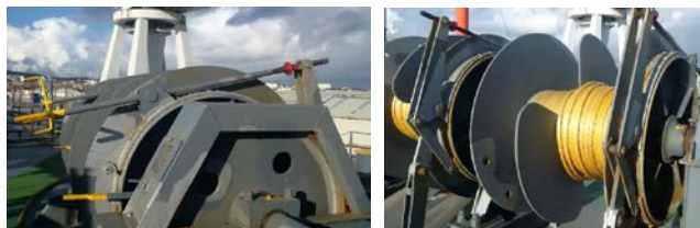
Figure 4. Conventionally screw manually-applied band brake of Crude Oil Tanker "Tulip".
