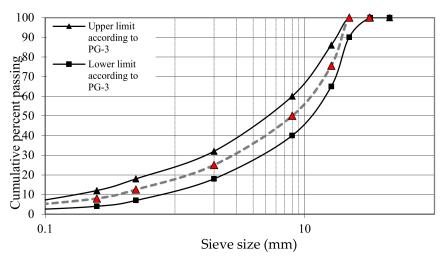
Figure 3. Gradation curve of AC-22 base G.
