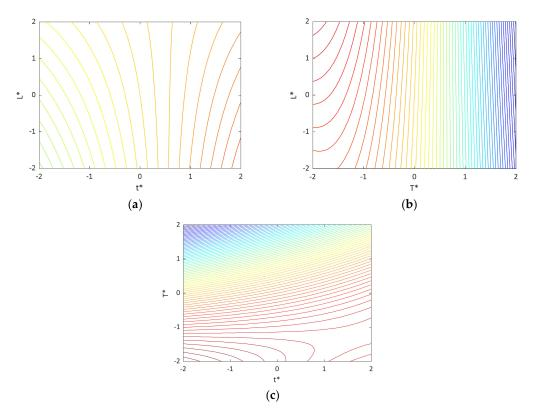
**Figure 7.** Contour plots of the  $ln(M_R)$  at the plane of two scaled predictor coordinates at the center of the excluded third one: (a) temperature (T\*) and binder content (L\*); (b) cure time (t\*) and binder content (L\*); (c) cure time (t\*) and temperature (T\*).
