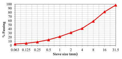
Figure 1. Gradation curve of recycled aggregate (RCA).
