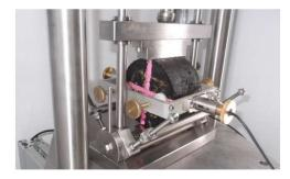
Figure 4. Resilient modulus test equipment.
