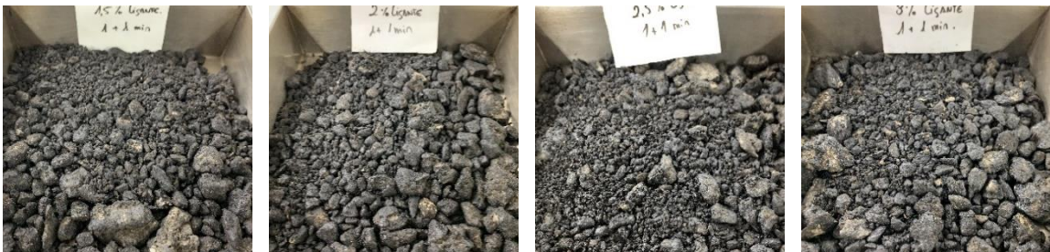
20 Figure 6 – Visual analysis of samples immediately after curing at 50 °C for 3 d using mixing time 1
