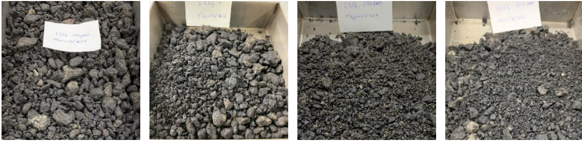
1 Figure 7 – Visual analysis of samples immediately after curing at 50 °C for 3 d using mixing time 2
