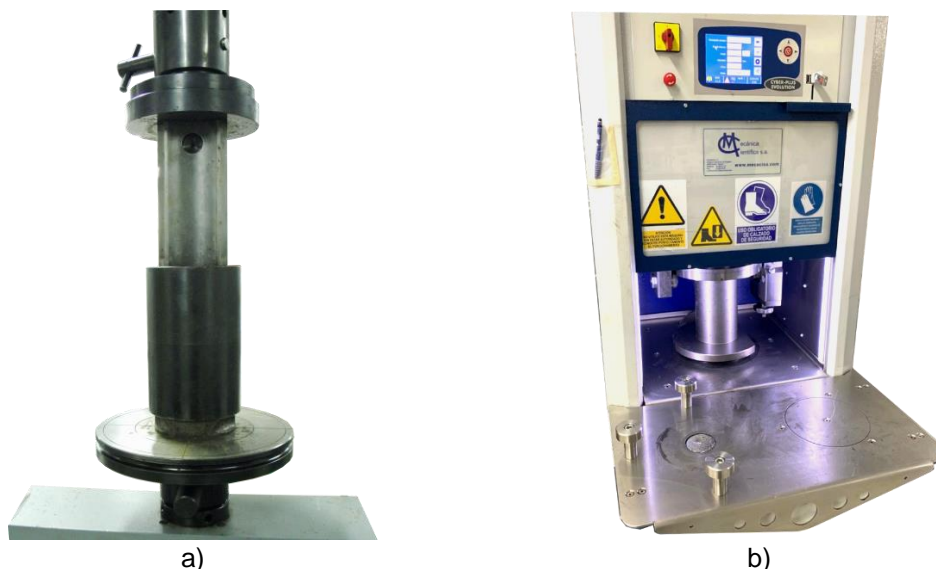
Figure 2 – Compaction equipment: a) static compactor; b) gyrotory compactor
