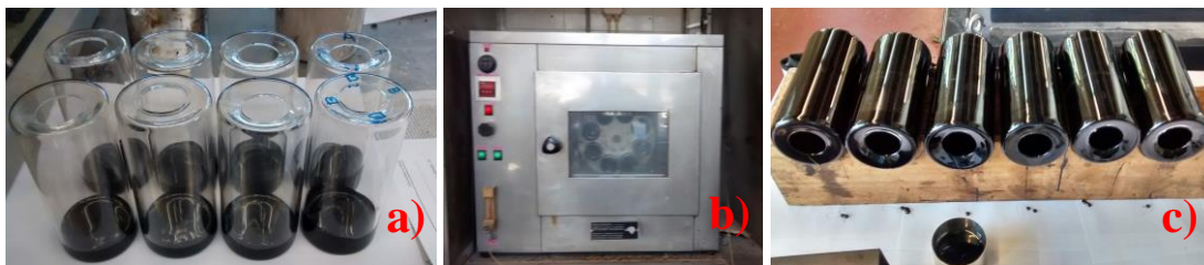
Fig. 2 RTFOT: a) bottles loaded with asphalt prior to ageing; b) bottles loaded with asphalt placed in oven; and c) bottles loaded with asphalt following ageing
