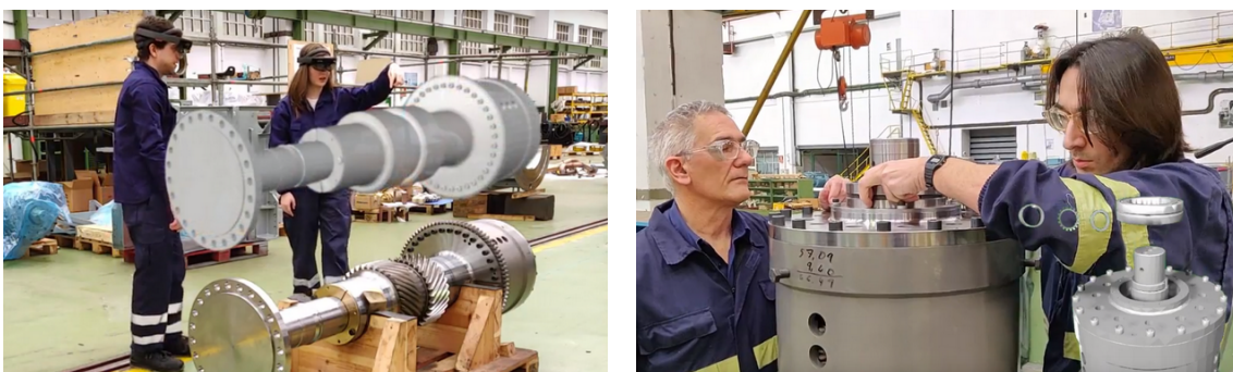
Figure 1. Interaction with the 3D model (left) and assembly process at Navantia's Turbine workshop (right).
