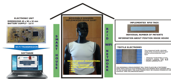
Figura 3: The scheme of the textronics system for protecting of elders. M. Frydrysiak and L. Tesiorowski, "Wearable textronic system for protecting elderly people," 2016 IEEE International Symposium on Medical Measurements and Applications (MeMeA), Benevento, 2016, pp. 1-6.
