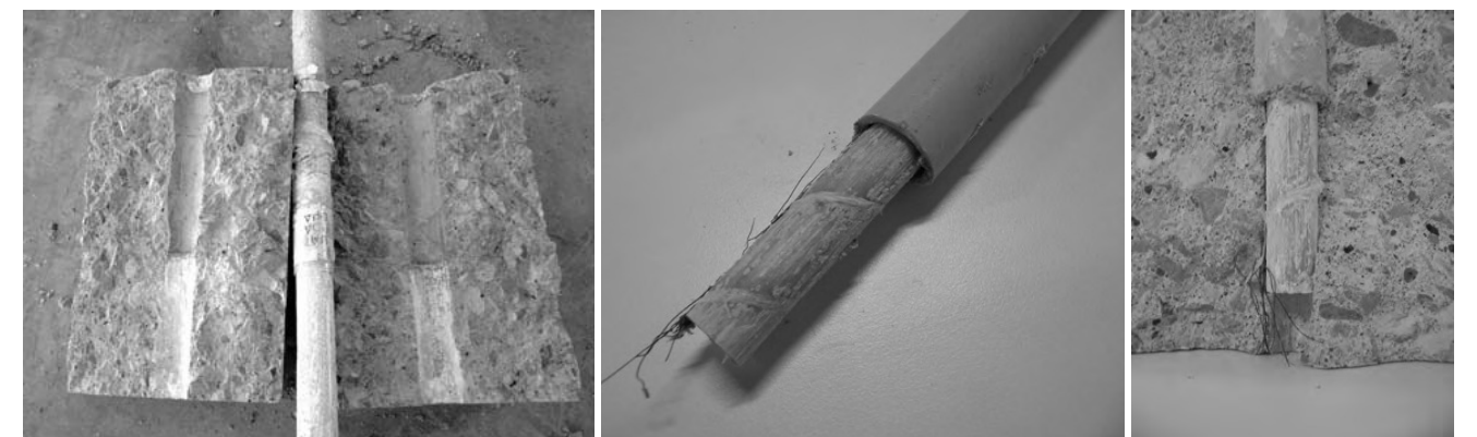
BAENA MUÑOZ, Marta. Pull out Test Results. "Study of bond behaviour between FRP reinforcement and concrete". Tesis doctoral.
