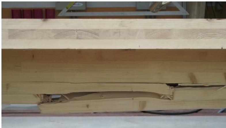
Fig. 13. Tensile failure in the Norway Spruce web due to the existence of knots.
