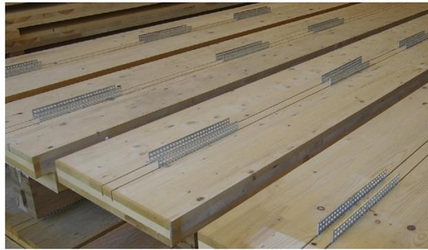
Fig. 2. Discontinuous connections on the top plank (separations between plates are described in Fig. 5).
