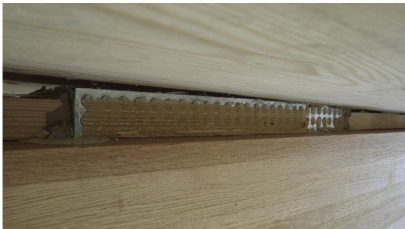
Fig. 11. Failure in the connection between the web and upper flange in a single unreinforced beam.
