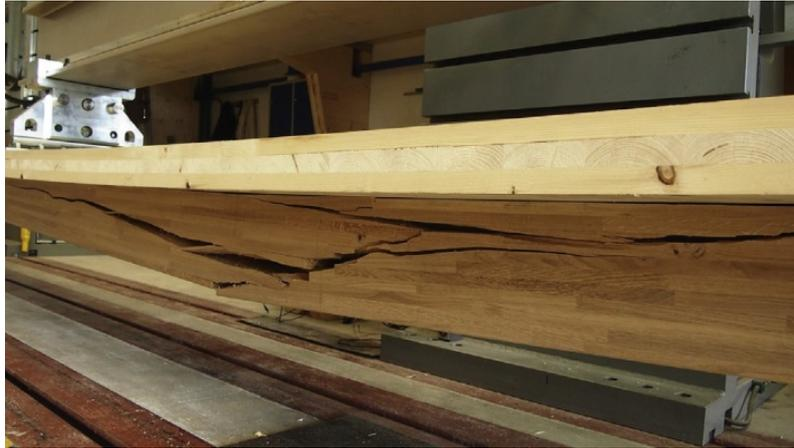
Fig. 12. Typical tensile failure initiated in the bottom laminations of the oak web.
