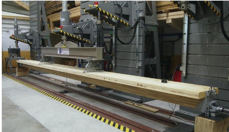
Fig. 6. Four-point bending test in the configuration with the self-tensioning device.
