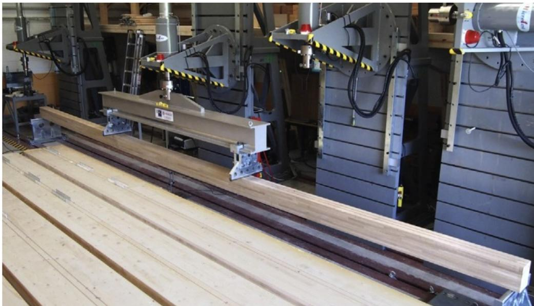
Fig. 4. Preliminary bending test (European Oak web).
