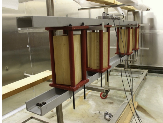
Fig. 6. Group of test specimens in preparation phase inside the climatic chamber.
