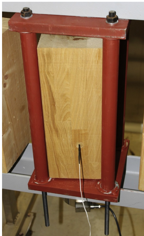
Fig. 3. Thermocouple inserted into the specimen (prior to sealing).
