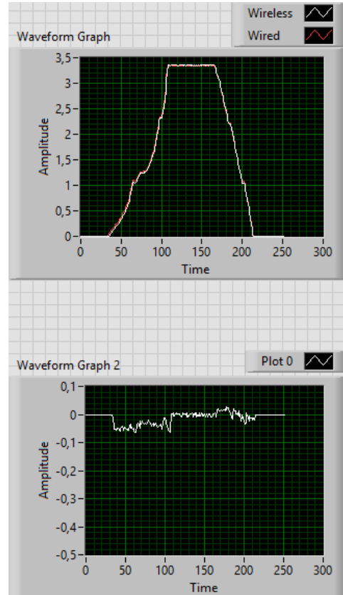
Fig. 7: Wireless (Arduino + XBee) vs. wired (NI myDAQ USB-6008). Top : Obtained signals. Bottom : Difference between the signals
