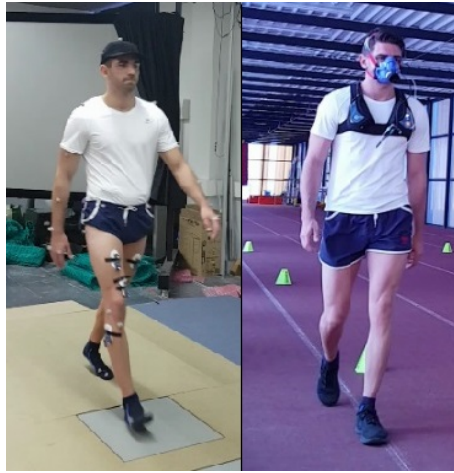
Figure 4.1 – Energy consumption for a healthy subject: a) motion-force-EMG capture; b) 5-minute test with portable gas analyzer.
