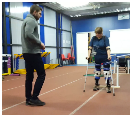
Figure 5.10 – Patient using the active orthoses with crutches.
