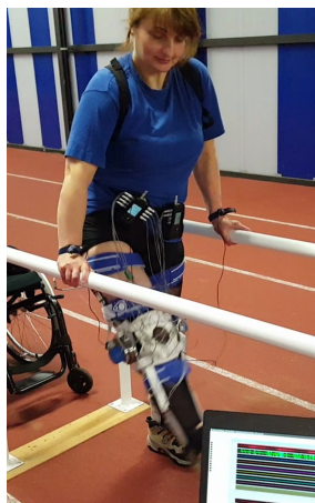
Figure 5.4 – Motor test with surface EMG to assess muscle activity.
