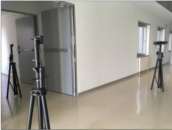
(a) Picture of the corridors showing two of the three anchors and the tag employed in the UWB measurement campaign.
