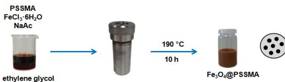
Figure 10. Scheme of the synthetic procedure and representation of a nanoparticle structure with \text{Fe}_3\text{O}_4 nanocrystals (black) embedded in PSSMA (grey).
