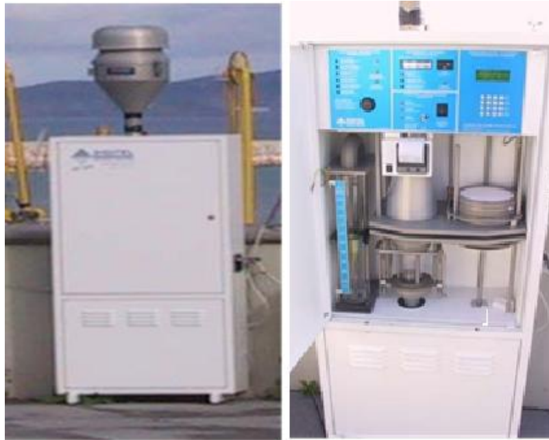
Figure 4. External and internal vision of the DHA-8 high-volume sampler.
