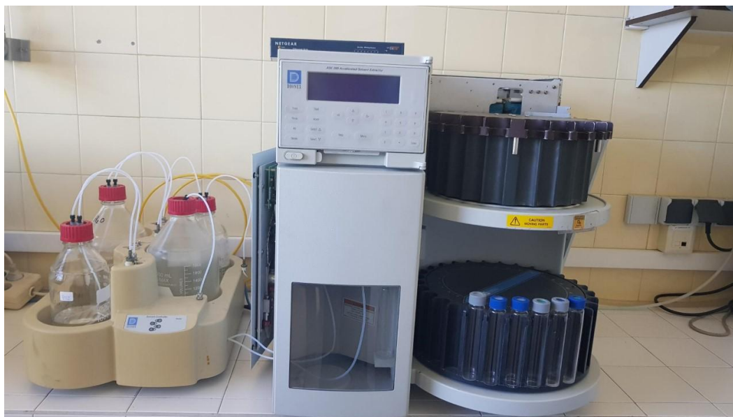
Figure 7. Illustration of the Accelerated Solvent Extractor Dionex ASE.
