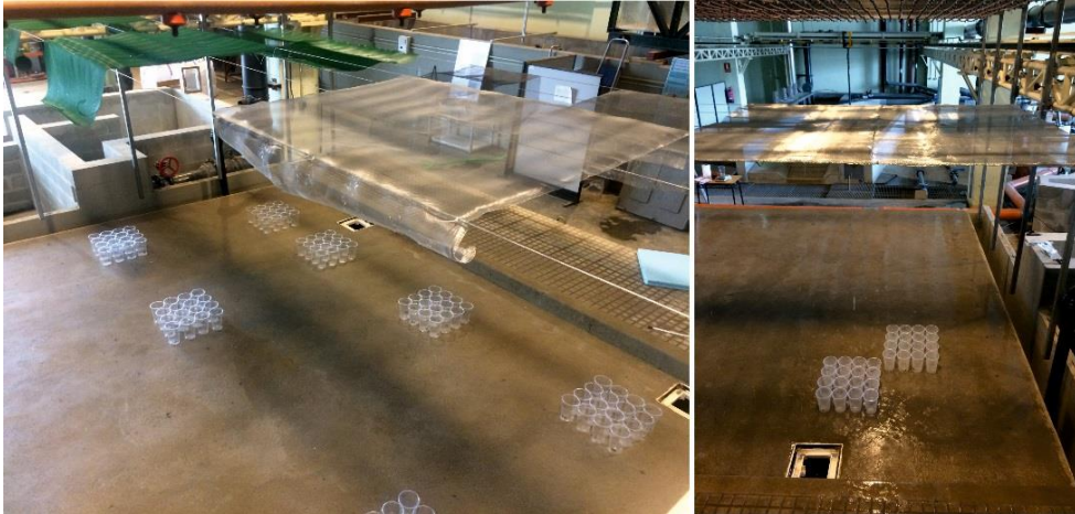
Figure 3.2. Vessels disposed over the model surface to measure rain intensity and uniformity for different mesh types and distances to drippers during calibration.
