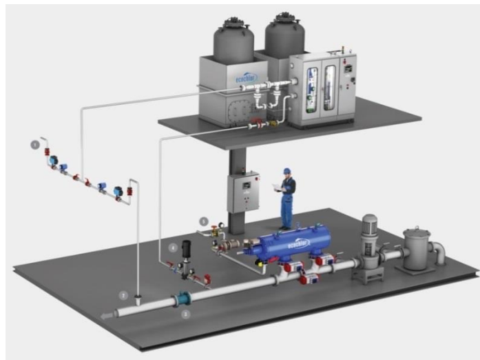
Figura 6.2.4.1.1 - Ecochlor Ballast Water Treatment System. Fuente: https://ecochlor.com/system/
