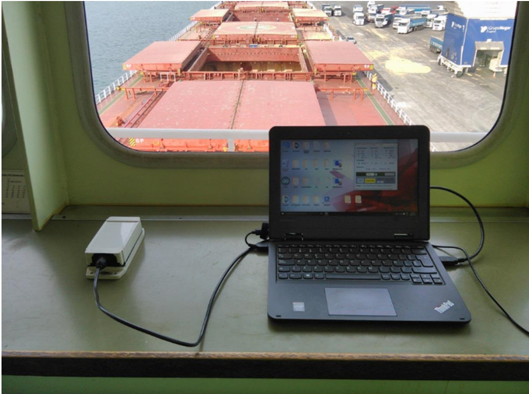
Fig. 4. IMU installed inside the vessel.
