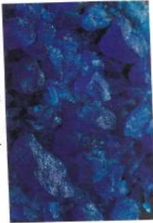
Figure 1 Copper sulfate crystals
