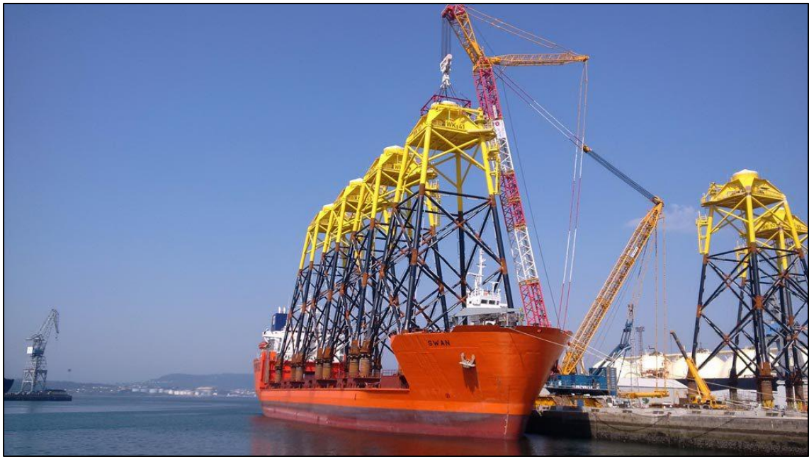
Figura 26. Load Out jackets Wikinger Astillero Navantia Fene
