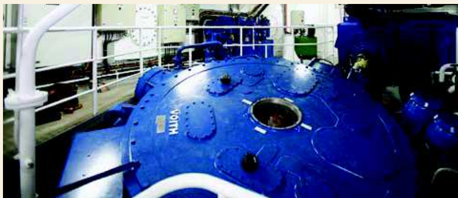
VSPs can generate propulsion and steering forces and be used to reduce roll
