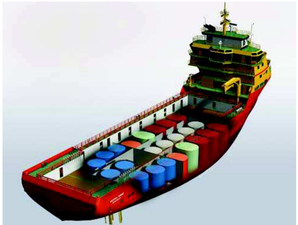
Edda Fram can carry a variety of cargoes and slops, including low flashpoint liquids
