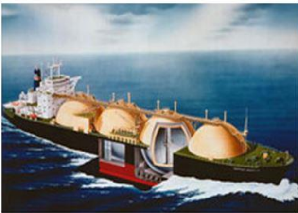
Section through Moss LNG vessel
