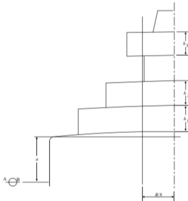
FIGURE 1 Effective Heights of Deck Houses
