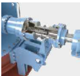
Disconnection of the drive shaft before the thruster is lifted up.
