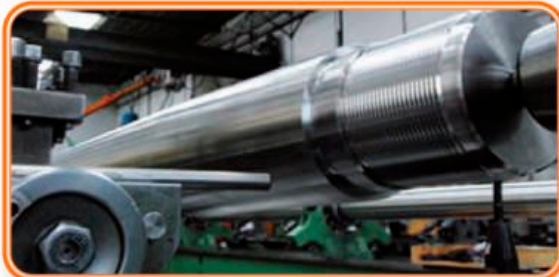
Lathe parts up to a total length of 16 m with cone and thread
