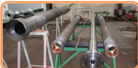
Pipes, stern tubes and shafts with forged flange
