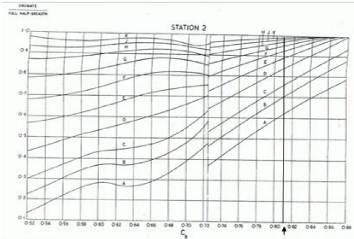
Fig. 36—Station 2. Waterline Offsets Expressed as the Ratio of Waterline Ordinate/Full Half-Breadth.
