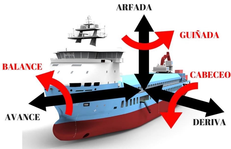
Figura 3.1. Grados de libertad de un buque. Fonte: ("DryTank Shipping – Shipping broker company," n.d.)
