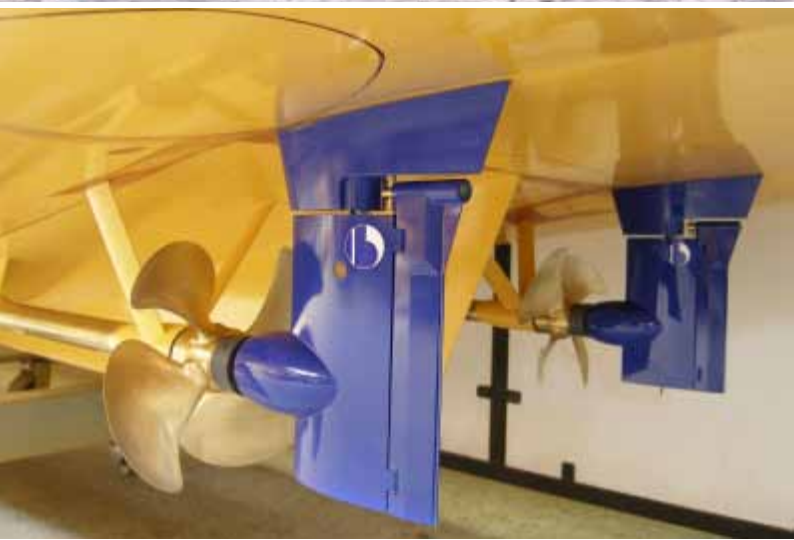
Energopac incorporated in model tests, photographed by HSVA.
