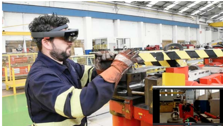
Figure 6. One of the tests in the pipe workshop with the HoloLens augmented collaboration application.
