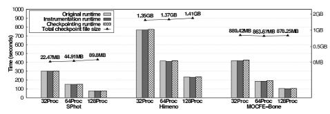
Fig. 5 Runtimes for the testbed benchmarks, specifying number of processes and total checkpoint file size.
