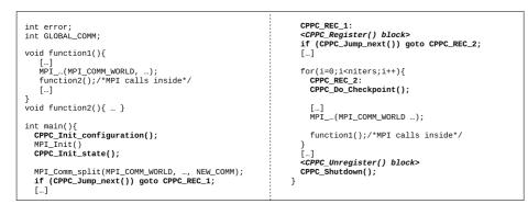
Fig. 1 CPPC instrumentation for stop and restart fault-tolerant applications.
