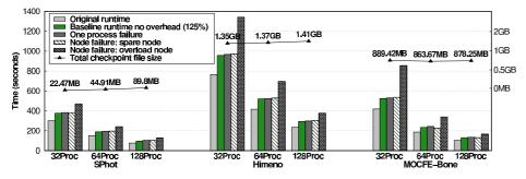
Fig. 7 Runtimes when introducing failures varying the number of processes. The baseline runtime in which no overhead is introduced is included for comparison purposes.
