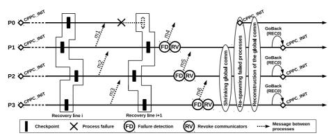
Fig. 2 Obtaining resilient MPI applications with CPPC and ULFM.
