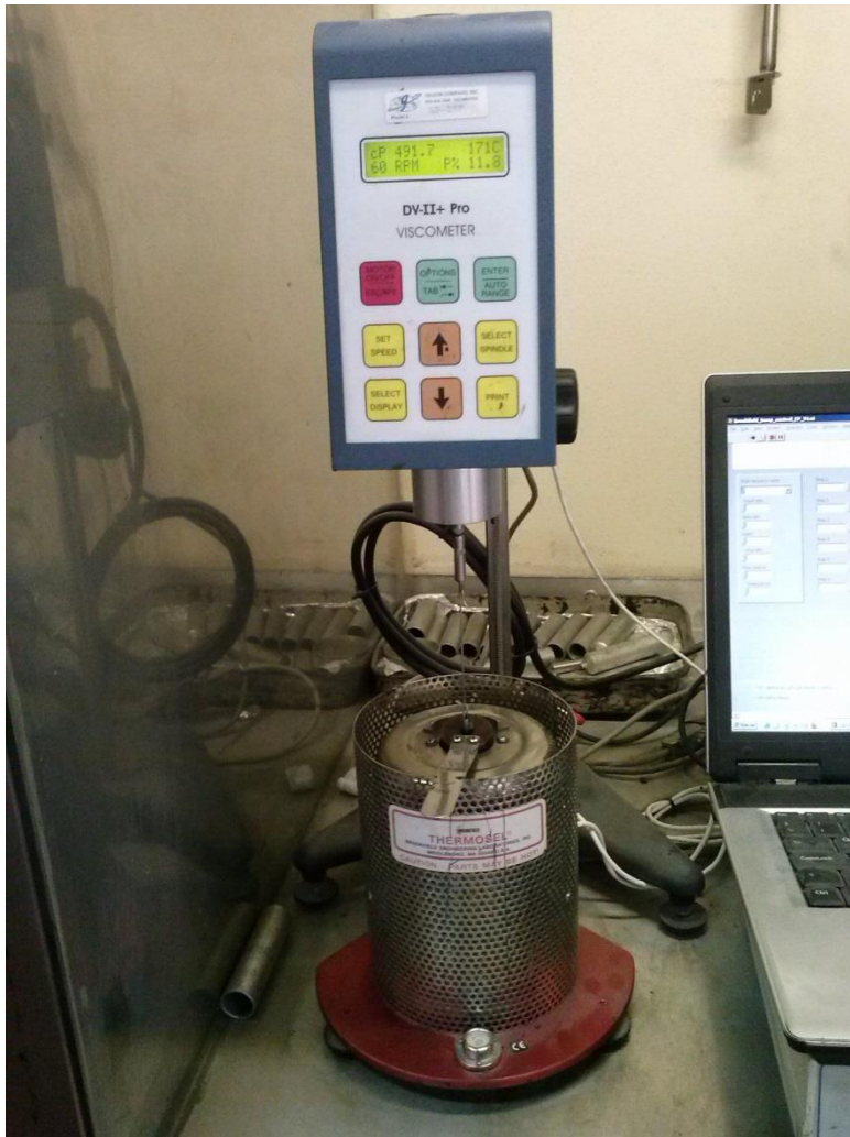
Figure 4. Rotating spindle apparatus used for the dynamic viscosity tests
