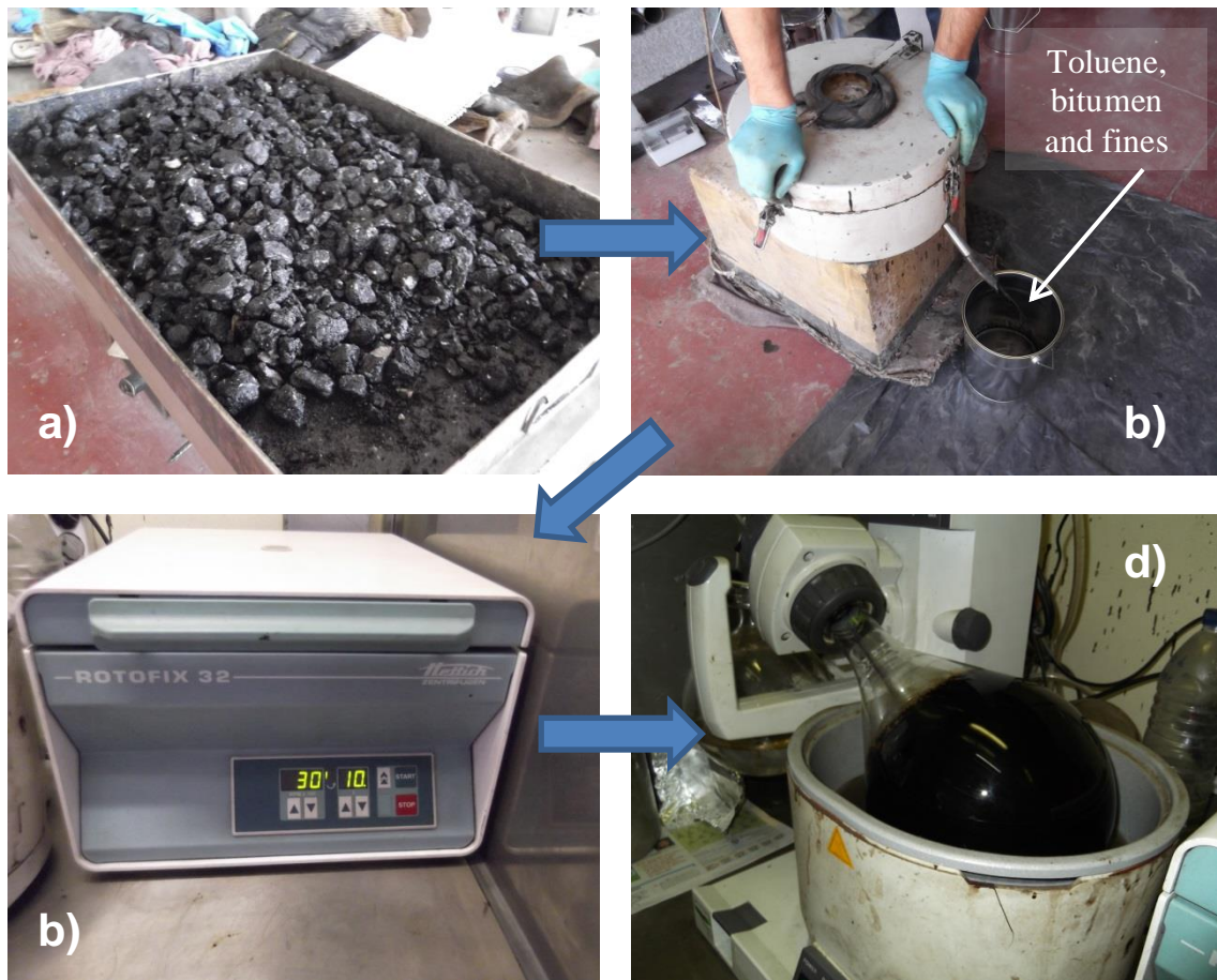
Figure 1. Bitumen recovery procedure: a) Loose asphalt mixture; b) Centrifuge extractor; c) Centrifuge used to decant fines from the solution of toluene, bitumen and fines and d) Rotary evaporator used to separate bitumen from toluene
