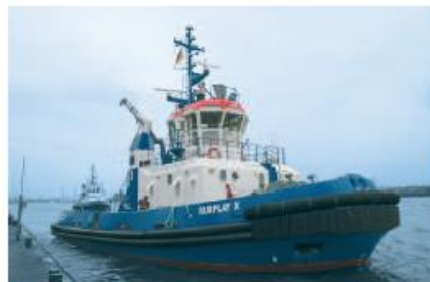
64 T BP ASD TUG FAIRPLAY X 2 x SCHOTTEL Rudderpropeller Type SRP 1515 FP (1865 kW each)
