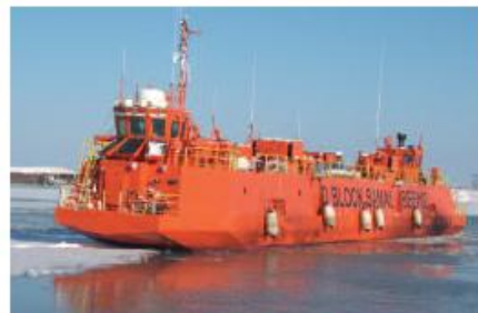
ICEBREAKING EMERGENCY EVACUATION VESSEL IBEEV 02 2 x SCHOTTEL Rudderpropeller Type SRP 550 PULL (560 kW each)
