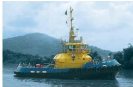
45 T BP ASD TUG SMIT TUPI 2 x SCHOTTEL Rudderpropeller Type SRP 1012 FP (1378 kW each)
