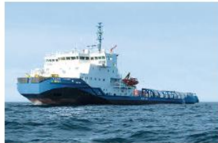
ICE BREAKING MULTI-PURPOSE VESSEL TULPAR 2 x SCHOTTEL Rudderpropeller Type SRP 2020 PULL (2000 kW each)
