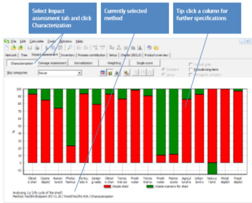
Figure 34: Results of the characterization step. All impact scores are displayed on a 100% scale. The colors indicate the contribution of production and waste.
