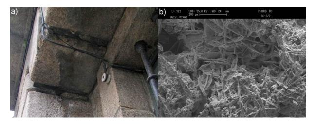
Figure 5. Example of carbonate crusts on granite stones.
